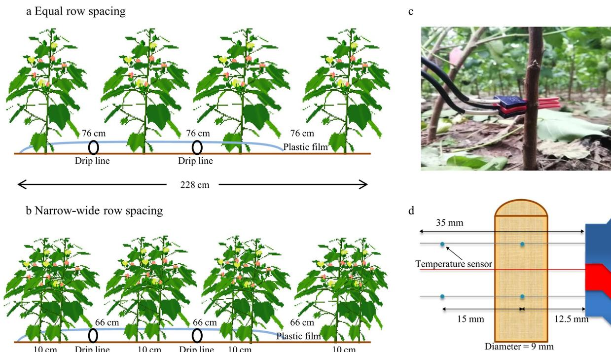
**Fig. 2** Row configurations of the field experiment (a, b) and the installation of sap flow meter (c, d)
