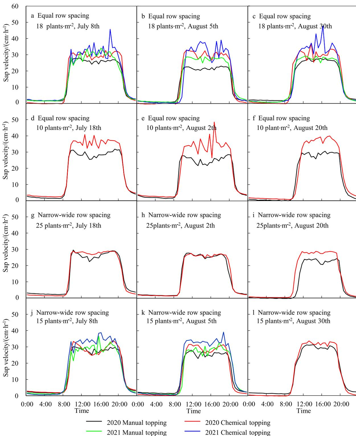
**Fig. 5** Diurnal courses of sap velocity in three sunny days at different development stages under different row configurations (equal row spacing, narrow-wide row spacing), plant densities and topping treatments in 2020 and 2021
